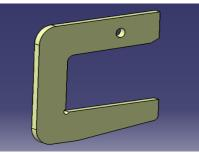
Figure 4: C frame of balanced c-hook.
