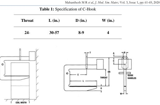
Figure 2: Balanced C-Chook with Coil and Specification Sketch.
