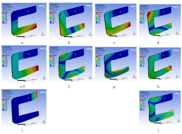
Figure 11: Mode shapes for ASTM Grade 60
