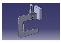
Figure 3: balanced c-hook assembly.
