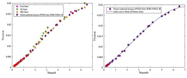
Fig. 20: Multi-objective optimization results by NSGA-II.
