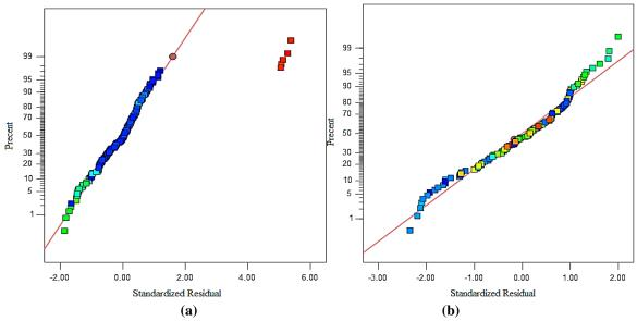
Fig. 16: Normal probability plot residuals. (a) Friction (b) Nusselt
