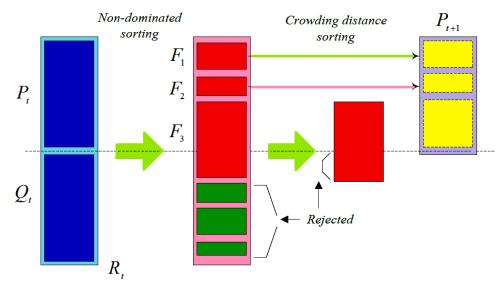
Figure 2: The structure of NSGA-II.
