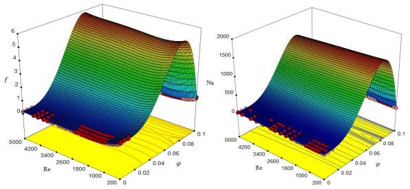
Fig. 18: Three-dimensional response surface graphs of Friction. Fig. 19: Three-dimensional response surface graphs of Nusselt.
