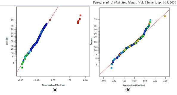
Fig. 10: Normal probability plot residuals. (a) Friction (b) Nusselt
