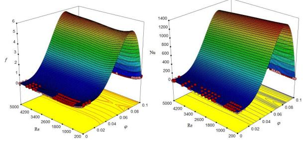
Fig. 12: Three-dimensional response surface graphs of Friction. Fig. 13: Three-dimensional response surface graphs of Nusselt.
