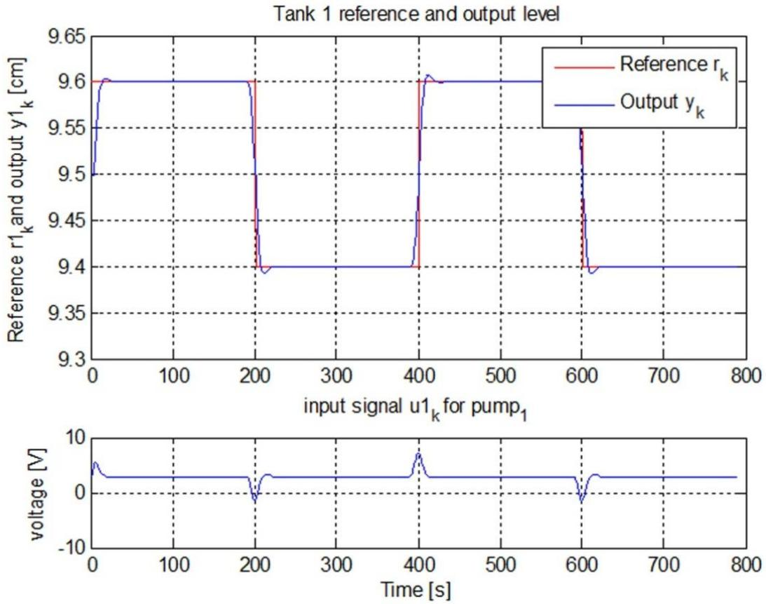
**Figure 1:** Unconstrained MPC controller response for tank 1. The upper two plots illustrated the reference signal and output levels for tank 1. The lower plot is the controller input signal for pumps 1.
