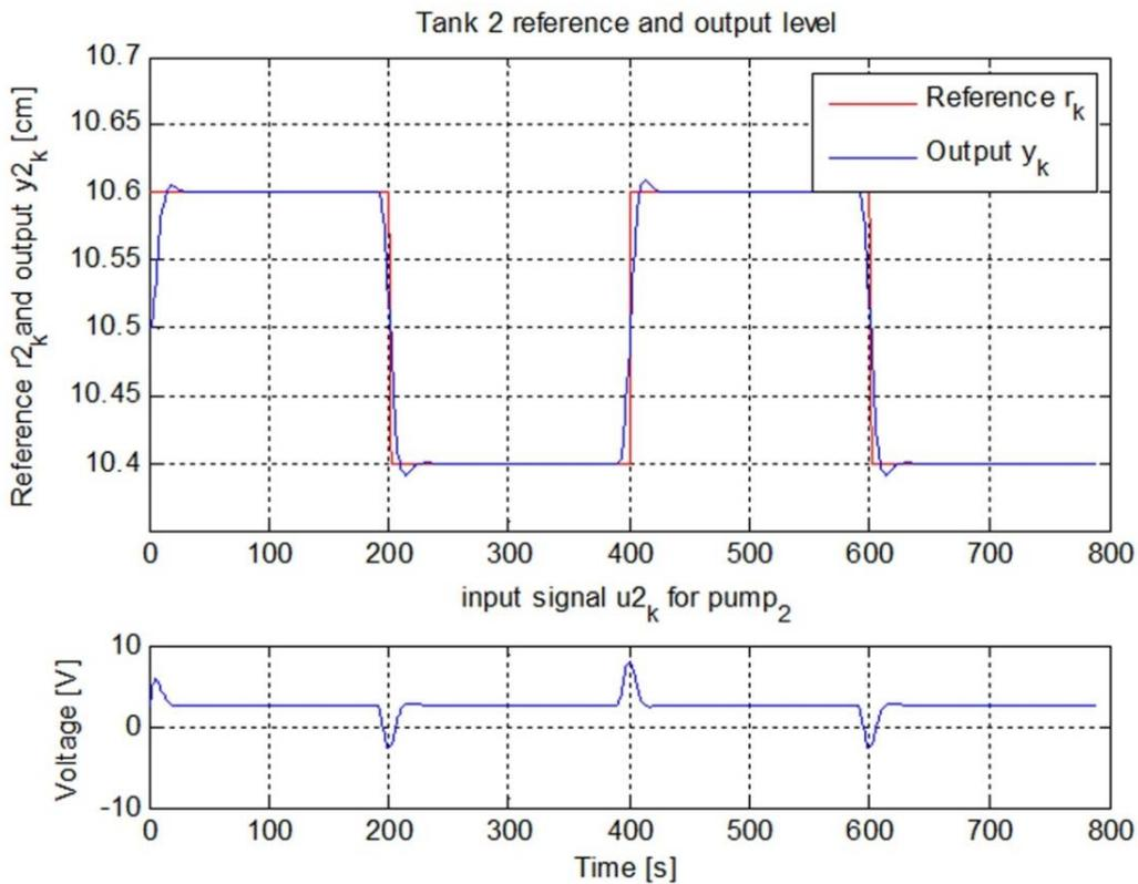
**Figure 2:** Unconstrained MPC controller response for tank 2. The upper two plots illustrated the reference signal and output levels for tank 2. The lower plot is the controller input signal for pumps 1.
