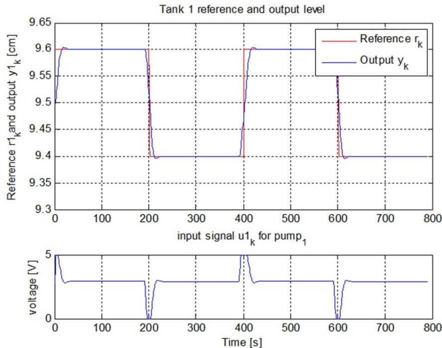
**Figure 3:** Constrained MPC controller response for tank 1. The upper two plots illustrated the reference signal and output levels for tank 1. The lower plot is the controller input signal for pumps 1.
