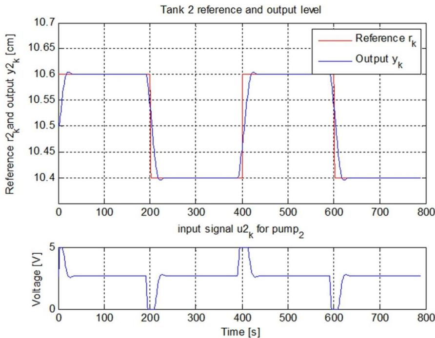
**Figure 4:** Constrained MPC controller response for tank 2. The upper two plots illustrated the reference signal and output levels for tank 2. The lower plot is the controller input signal for pumps 1.
