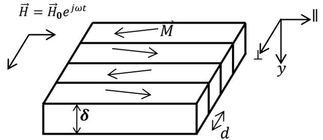
**Figure 1:** Wall domains in a ferromagnetic material
