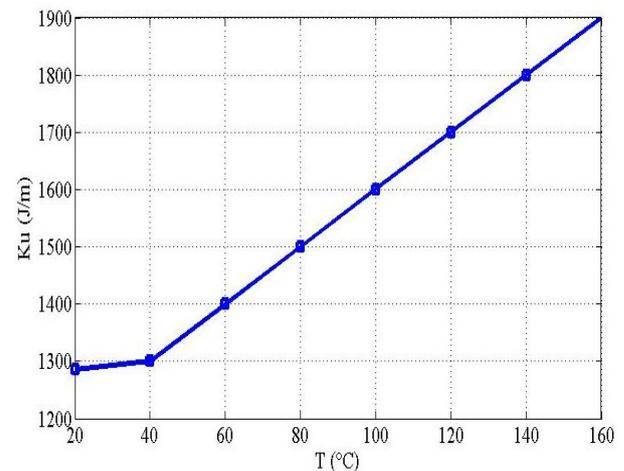
**Figure 10:** Variations of anisotropy energy with the temperature
