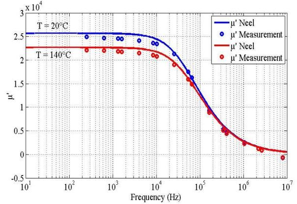
**Figure 7:** Real part of the complex permeability versus the frequency at  $T=20$  °C and  $T=140$  °C
