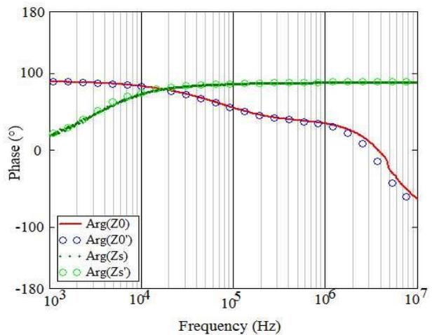
**Figure 5:** Open and short circuit impedance arguments at 40 °C
