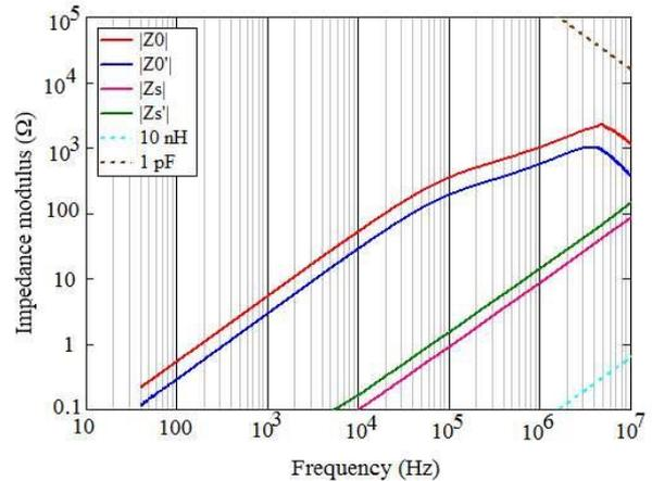
**Figure 4:** Open and short circuit impedance modulus at 40 °C
