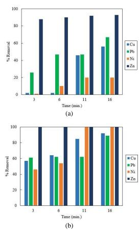
**Figure 4**: Percentage (%) removal of Cu, Pb, Ni and Zn with respect to the time at (a) 1<sup>st</sup> collection point and (b) 2<sup>nd</sup> collection point
