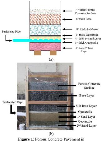
(a) Schematic View and (b) Model
