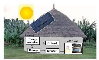
Figure 4: The block diagram of the household stand-alone PV system
