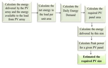
Figure 2: Schematic diagram for sizing Solar panels
