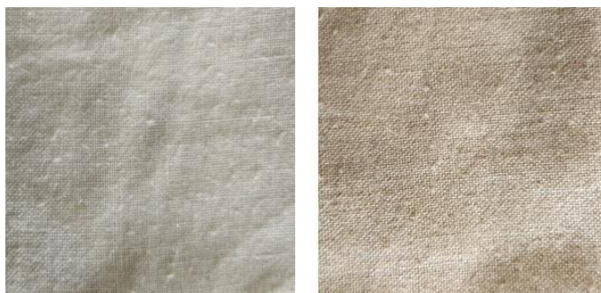
Figure 12: Optical images of (a) untreated cotton cloth and (b) cloth treated with AgNPs made from tea extract
