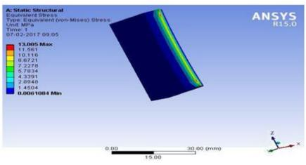
Figure 10: Analysis of cutting blades in ANSYS 15
